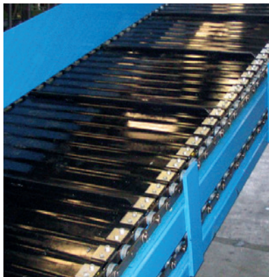
Steel plate conveyor
